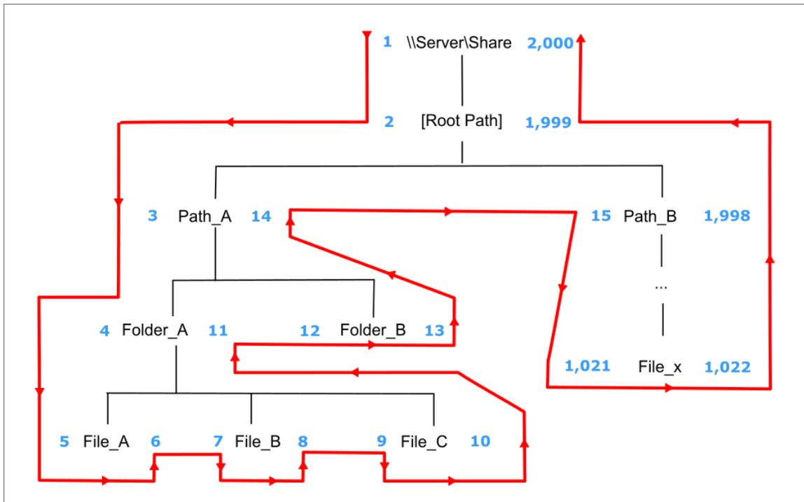
For each node in the scanned file structure, a left (*ns\_left*) and right (*ns\_right*) value are assigned. The values are assigned by traversing the imaginary path from the root down the left side of the structure, incrementing the *ns\_left* values by one. Once a leaf node is encountered, the incrementing value continues, but is now assigned to *ns\_right*.
